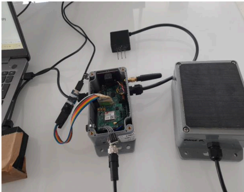
Connecting the serial cable between the TTCyber and your PC
